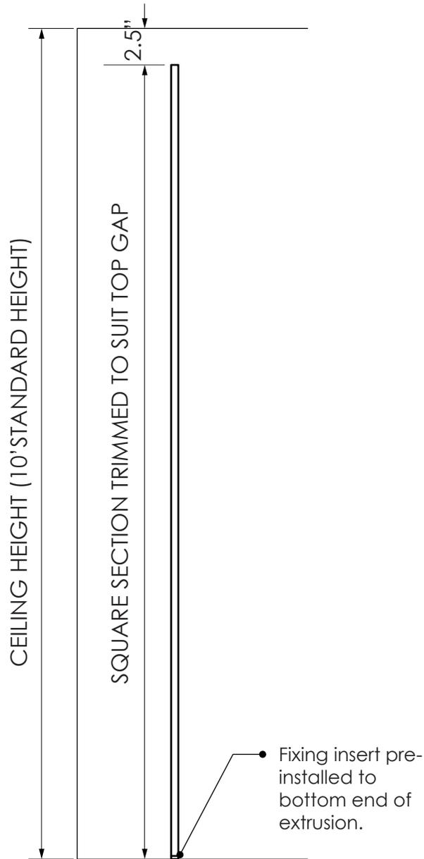
2) Knock-in fixing insert to open end of extrusion.
