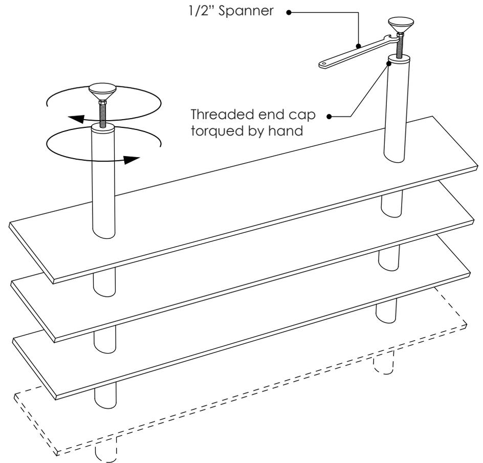
9) Screw out tensioner to compress louver assembly into cavity & then sandwich spacers with threaded end cap by screwing down.
