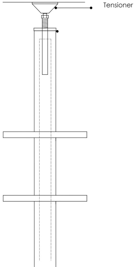
10) Ensure level before fixing off base plate to floor with appropriate fastener for application.
