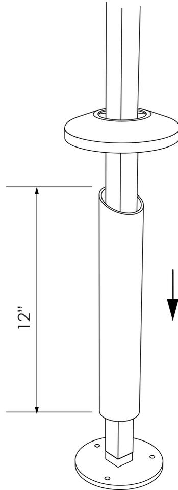
6) Sleeve louver & spacer tubes. Repeat as required.
