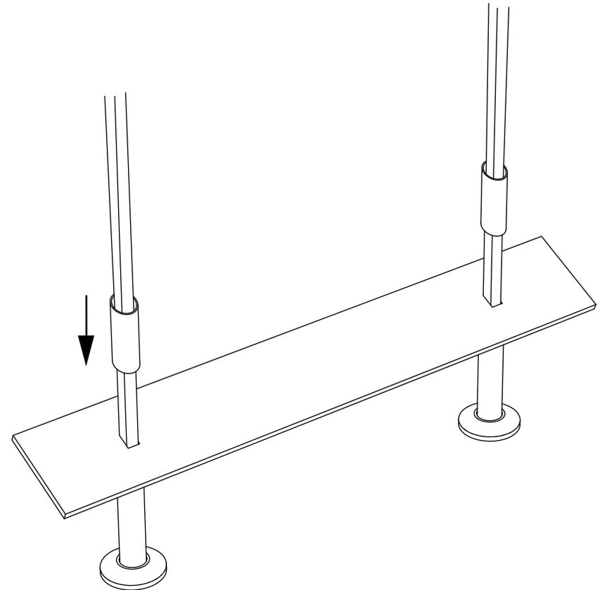
7) Screw in tensioner to top extrusion with threaded end cap.
